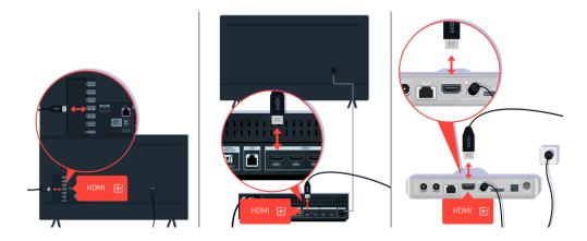
Check the antenna and HDMI cable connections.
