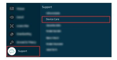
Go to a >  $\equiv$  Menu > s Settings > Support > Device Care > Self Diagnosis > Sound Test to check the sound.
