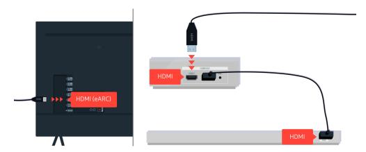
If your Sound Bar is connected to a receiver, and the receiver is connected to the TV using an HDMI cable, check the HDMI connector on the back of the TV. The cable must be connected to the HDMI (eARC) port on your TV.
