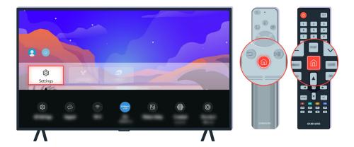
Go to a >  $\equiv$  Menu > s Settings > Support > Device Care > Self Diagnosis > Sound Test to check the sound.
