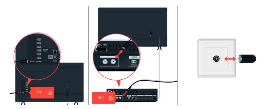
Check the antenna and input cable connections.
