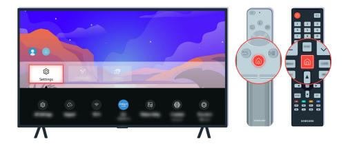
Select a >  $\equiv$  Menu > s Settings > Support > About This TV and check the model code and software version.
