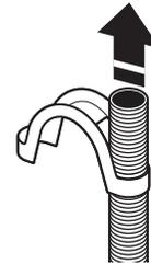
Bend drain hose over drain hose form and snap into place.
