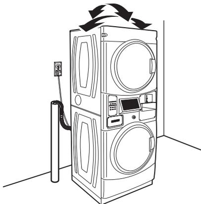
3. If washer/dryer is not level, use a 9/16" or 14 mm openend or adjustable wrench to turn jam nuts clockwise (as viewed from above) on feet until they are about 1/2" (13 mm) from the washer/dryer cabinet. Then turn the leveling foot counterclockwise to lower the washer/dryer or clockwise to raise the washer/dryer. Recheck levelness of washer/dryer and that all four feet are firmly in contact with the floor. Repeat as needed.
