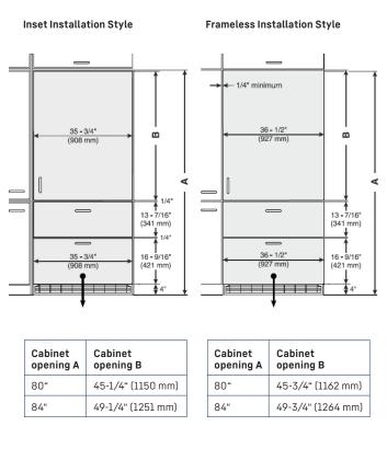
Minimum panel thickness is 5/8" (16 mm).
