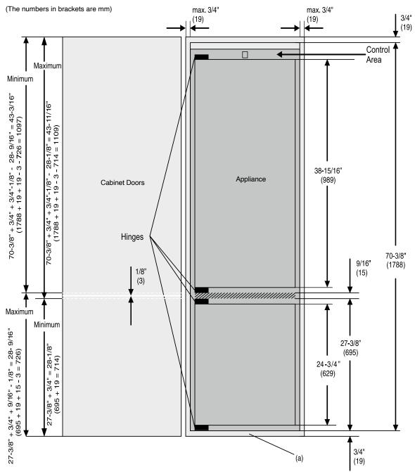
(a) The base of the cabinet can be thickened to raise the the top of the lower door panel to counter height. Lower panel will have to be increased in length by the same amount.
