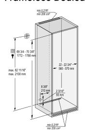
This is a fully integrated wine appliance designed to be completely enclosed in a dedicated kitchen cabinet. This dedicated cabinet box must be constructed in accordance with the specified dimensions and must allow for sufficient air circulation to ensure proper operation. For more details about ventilation requirements, please refer to page 42.
