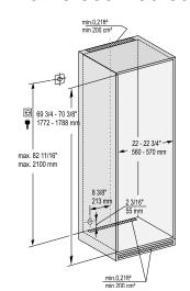
This is a fully integrated refrigerator appliance designed to be completely enclosed in a dedicated kitchen cabinet. This dedicated cabinet box must be constructed in accordance with the specified dimensions and must allow for sufficient air circulation to ensure proper operation. For more details about ventilation requirements, please refer to page 42.
