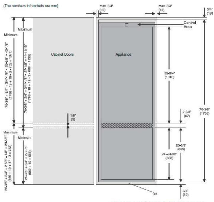
(a) The base of the cabinet can be thickened to raise the the top of the lower door panel to counter height. Lower panel will have to be increased in length by the same amount.
