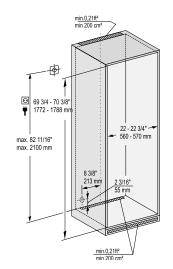
This is a fully integrated refrigerator-freezer appliance designed to be completely enclosed in a dedicated kitchen cabinet. This dedicated cabinet box must be constructed in accordance with the specified dimensions and must allow for sufficient air circulation to ensure proper operation. For more details about ventilation requirements, please refer to page 42.
