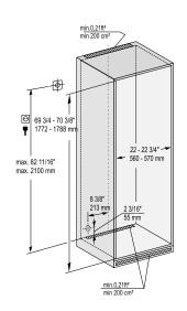
This is a fully integrated refrigerator-freezer appliance designed to be completely enclosed in a dedicated kitchen cabinet. This dedicated cabinet box must be constructed in accordance with the specified dimensions and must allow for sufficient air circulation to ensure proper operation. For more details about ventilation requirements, please refer to page 42.
