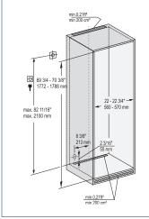
This is a fully integrated refrigerator-freezer appliance designed to be completely enclosed in a dedicated kitchen cabinet. This dedicated cabinet box must be constructed in accordance with the specified dimensions and must allow for sufficient air circulation to ensure proper operation. For more details about ventilation requirements, please refer to the Design Guide.
