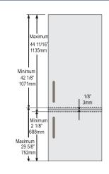
This is a sliding door model, which means the doors of the appliance are installed on the hinges of the dedicated box cabinet doors.
