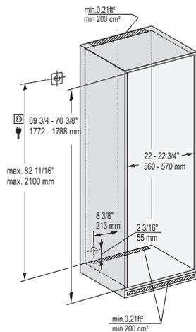
This is a fully integrated refrigerator appliance designed to be completely enclosed in a dedicated kitchen cabinet. This dedicated cabinet box must be constructed in accordance with the specified dimensions and must allow for sufficient air circulation to ensure proper operation. For more details about ventilation requirements, please refer to Design Guide.
