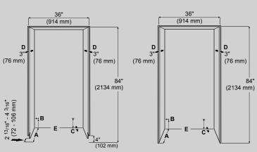
Cabinet depth frameless installation style = 25" (635 mm) Cabinet depth inset installation style = 25" (635 mm) + panel thickness
