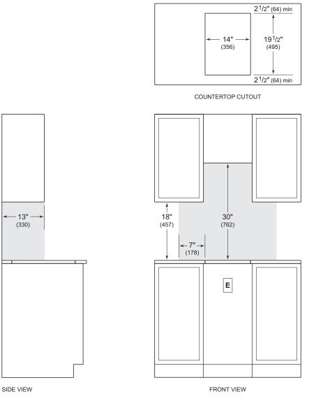
NOTE: Shaded area above countertop indicates minimum clearance to combustible surfaces, combustible materials cannot be located within this area.
