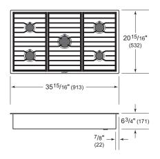
A minimum 2" (51) is required from the bottom of the cooktop to combustible materials. If the cooktop is installed above an oven, a minimum of 1/4" (6) is required between the units.
