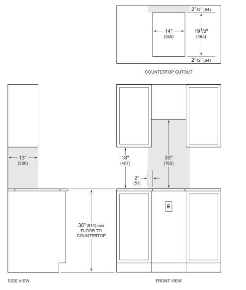
NOTE: Shaded area above countertop indicates minimum clearance to combustible surfaces, combustible materials cannot be located within this area.
