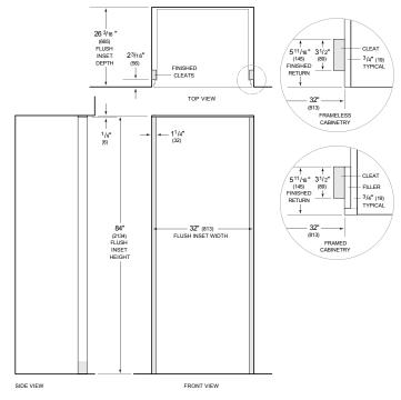
NOTE:  $3^1 k^n$  (89) finished returns and shaded areas will be visible and should be finished to match cabinetry Shaded line represents profile of unit  $\mathbf{w}^n k^n$  (19) panel.
