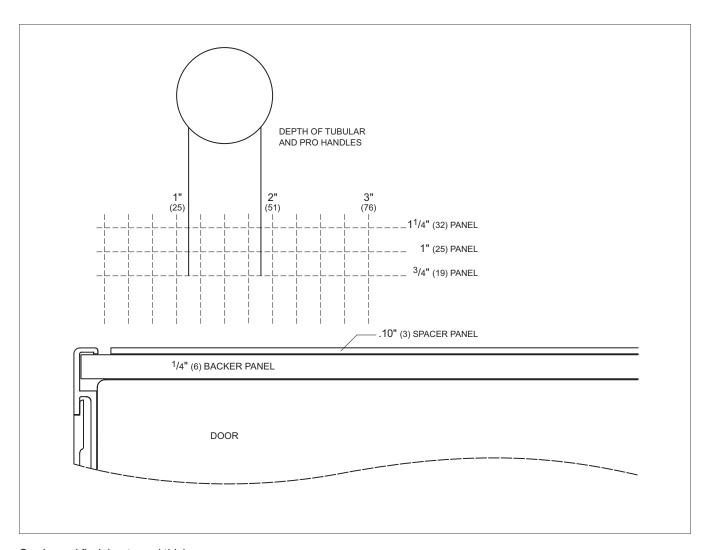
Overlay and flush inset panel thickness
