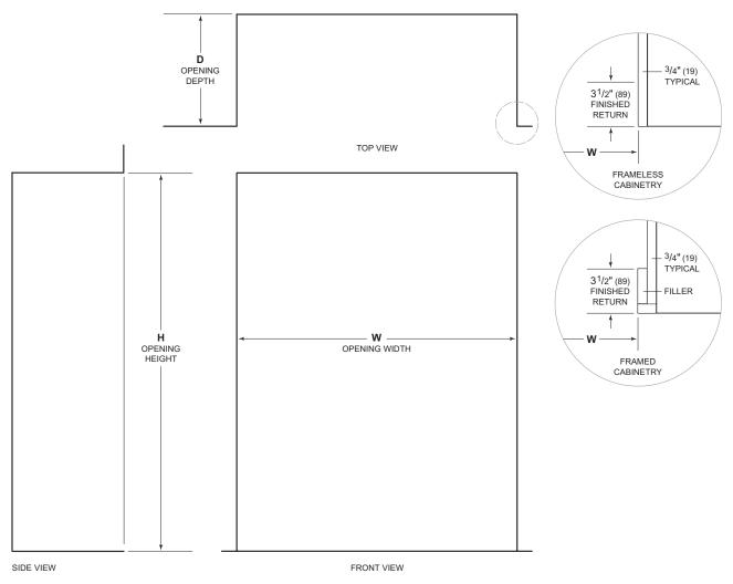
NOTE: 31/2" (89) finished returns will be visible and should be finished to match cabinetry.
