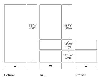
Typical panel dimensions are based on an 84" (2134) finished height for column and tall models and  $34\frac{1}{2}$ " (876) for drawer models, with a 4" (102) toe kick and  $\frac{1}{8}$ " (3) reveals. Panel dimensions must be adjusted accordingly for all other installations. Refer to the illustration for panel height and the chart below for panel width.
