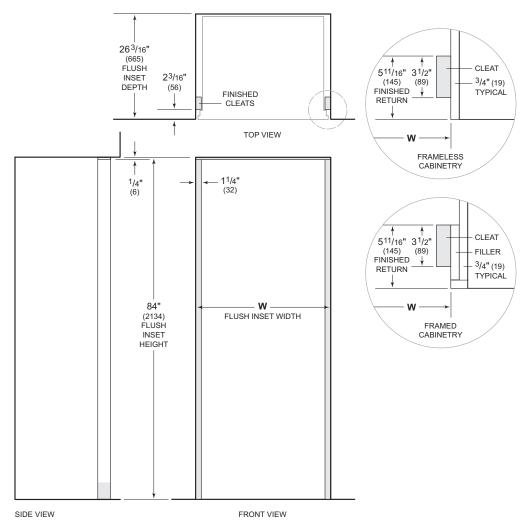
NOTE: 3<sup>1</sup>/2" (89) finished returns and shaded areas will be visible and should be finished to match cabinetry. Shaded line represents profile of unit with  $\,^3/4"$  (19) panel.
