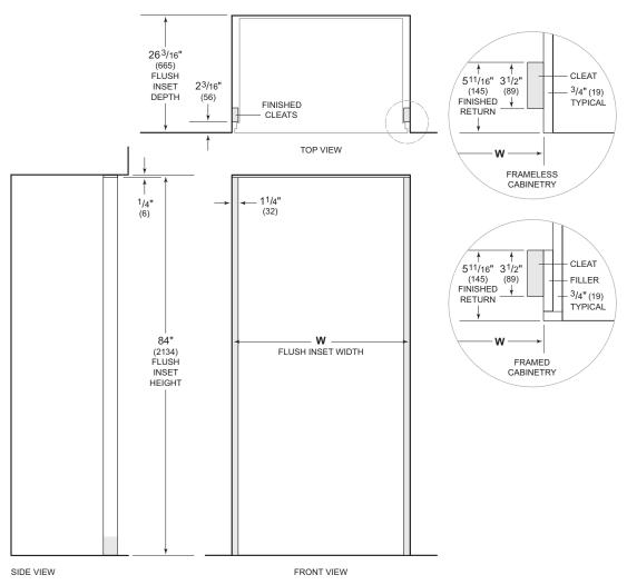
NOTE: 3<sup>1</sup>/2" (89) finished returns and shaded areas will be visible and should be finished to match cabinetry. Shaded line represents profile of unit with  $\,^3/4"$  (19) panel.
