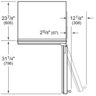
IMPORTANT NOTE: Overall dimensions are based on the stainless steel model. For flush inset applications, add ½" (13) to door clearance dimensions.
