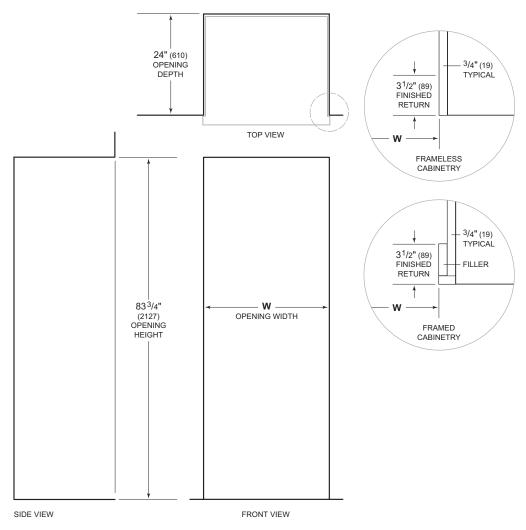
NOTE: 3<sup>1</sup>/2" (89) finished returns will be visible and should be finished to match cabinetry. Shaded line represents profile of unit.
