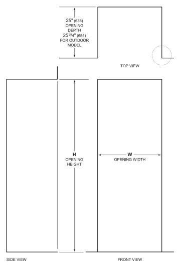
NOTE: 31/2" (89) finished returns will be visible and should be finished to match cabinetry— 41/2" (114) for outdoor model.
