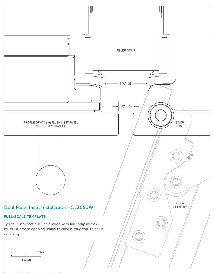
Dual flush inset installation (top view)
