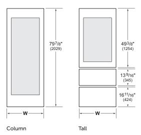
Typical panel dimensions are based on an 84" (2134) finished height, 4" (102) toe kick, and 1/8" (3) reveals. Panel dimensions must be adjusted accordingly for all other installations. Refer to the illustration for panel height and the chart below for panel width.
