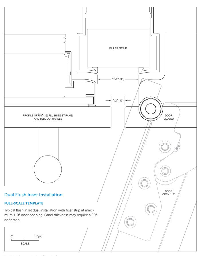
Dual flush inset installation (top view)
