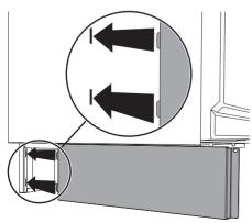
4. Line up the hole on the side skirting with the rear hole on the base of the appliance.
