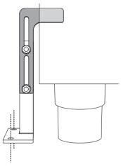
4. Lower the bracket attachment until anchoring the appliance slot, tighten the nuts previously assembled. The anti-tip device works properly only if the bracket attachment is securely anchored to the appliance.
