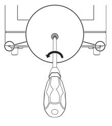
2. Position the front skirting at the bottom of the appliance and line up the side holes of the front skirting with the holes on the base of the appliance.
