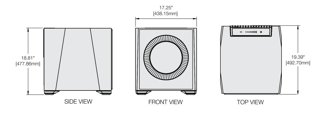
OVERALL DIMENSIONS\*: (H) 18.81" [477.86mm] x (W) 17.25" [438.15mm] x (D) 19.39" [492.7mm] WEIGHT: 103.8lbs (47.1kg) each
