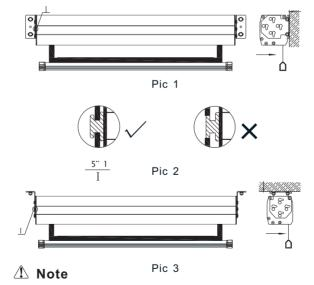
Please keep the screen casing and assembling plates in horizontal direction and install firmly (Pic 2).
