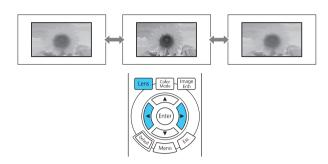
3 Press the Lens button on the remote control again and use the ◀ and ► buttons to reduce or enlarge the image.
