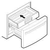
**5** Replace the ice bin(s) in the drawer. Insert the Durabase basket in the rail assembly.
