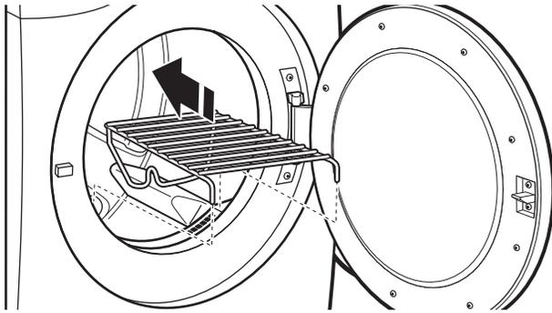
2. Align the two hooks on the front of the drying rack with the holes in the dryer door opening and press down fully into holes. Rest the rear support on the dryer back ledge.
