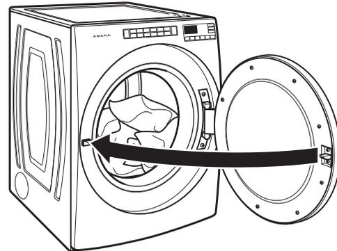
Open the door by pulling on the handle. Place laundry in the dryer. Add a dryer sheet to wet load, if desired. Close the door. **IMPORTANT:** Do not tightly pack the dryer. Items need to tumble freely. Tightly packing can lead to poor drying performance and may increase wrinkling and tangling.
