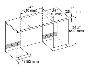
A: Recommended area for installation connection - a 2<sup>1</sup>/2" (63 mm) diameter hole is recommended. Location of power cord at base of the appliance.
