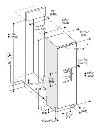
The door face dimensions are designed for a maximum gap of  $\ensuremath{\,^{\sc vs}}$  (3 mm).
