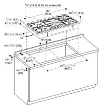
Minimum distance from the appliance cut-out to the side wall 11 (3/06/ mm).
