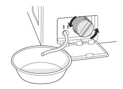
**5** Clean the pump filter and opening.
