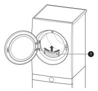
Always ensure the lint filter is properly installed before running the dryer. Running the dryer with a loose or missing lint filter will damage the dryer and articles in the dryer.
