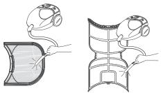
**3** If the lint filter has become very dirty or clogged with fabric softener, wash the lint filter in warm, soapy water and allow it to dry thoroughly before reinstalling.
