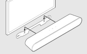
If your TV is wall-mounted, align the top edge of the bracket with the bottom of your TV, leaving at least 2.5 inches (mm) between them.
