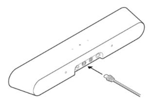
Connect the optical cable (included) to the optical port on the back of your soundbar.
