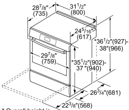
\* Overall height is adjustable via levelling legs.
