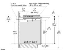
Dimensions based on standard countertop height (36" with  $43/4^{\rm m}$  toe kick including base plate).
