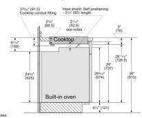
Dimensions based on standard countertop heigh (36" with 4<sup>3</sup>/<sub>4</sub>" toe kick including base plate).
