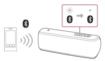
3. Press the WPC (Wireless Party Chain) button inside the cap on the rear side of the speaker.
