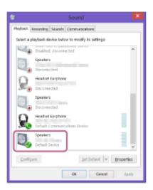
If you cannot click [Connect] for [SRS-XB31Stereo], select [Disable] for the [Default Device] that currently has a checkmark (green).
