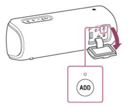
When you press and hold the ADD (Speaker Add) button, the voice guidance outputs from the speaker, then the mode changes.
