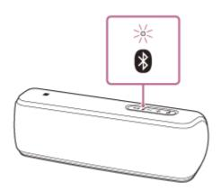
Perform the pairing procedure on the BLUETOOTH device to detect the speaker.
