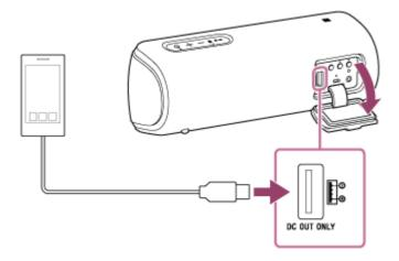
When you connect the speaker to an AC outlet, the connected USB device starts to be charged automatically. If the speaker is being powered by the built-in battery only, proceed to step ②.
