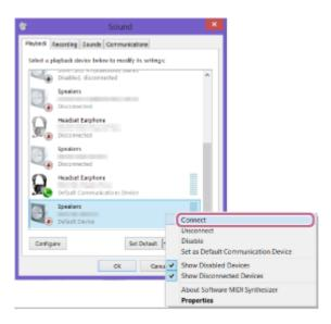
When the speaker is connected, a checkmark will appear on [SRS-XB31 Stereo] on the [Sound] screen. Proceed to step **6** .
