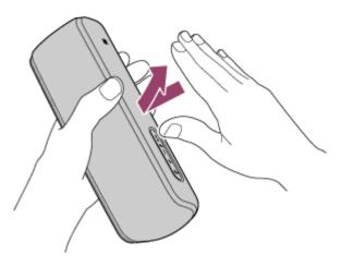
The surface where sound effects are output when you tap are the top, front, both sides, and bottom of the speaker.
