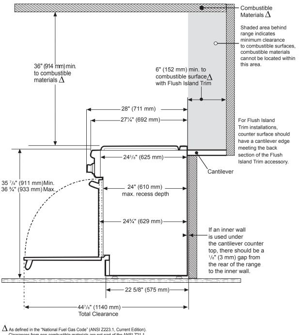
Clearances from non-combustible materials are not part of the ANSI Z21.1 scope and are not certified by CSA. Clearances of less than 6" (152 mm)
