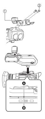
4 Slide the handle unit in the direction indicated by the arrow.
