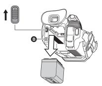
Move the battery release lever in the direction indicated by the arrow and remove the battery when unlocked.
