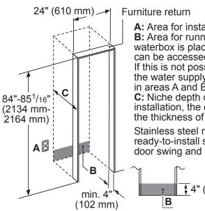
**A:** Area for installation of power connection.
