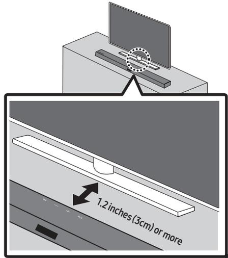
As illustrated in the image, align the center of the Soundbar with the center of the TV, carefully place the Soundbar onto the TV stand. For optimal sound quality, position the Soundbar at least 1.2 inches (3 cm) away from the TV front.
