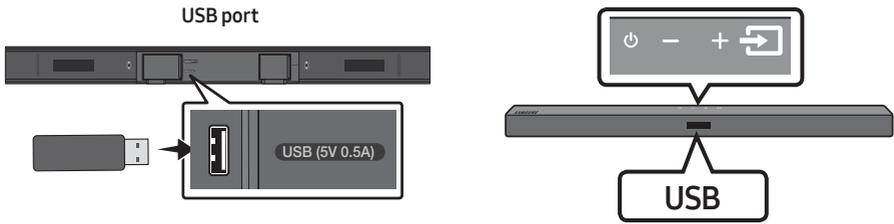
1. Connect the USB device to the USB port on the bottom of the product.
