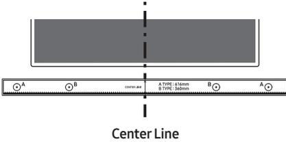
3. Push a pen tip or sharpened pencil tip through the center of the **B-TYPE** images on each end of the Guide to mark the holes for the supporting screws, and then remove the **Wall Mount Guide**.
