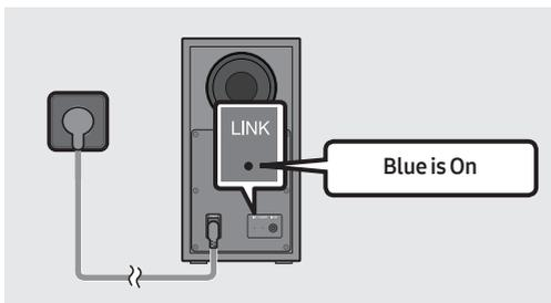
The LINK LED indicator stops blinking and glows a solid blue when a connection is established between the Soundbar and the Wireless Subwoofer.
