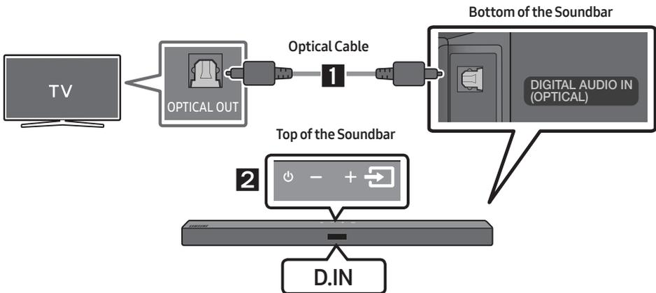
1. Connect the **DIGITAL AUDIO IN (OPTICAL)** port on the Soundbar to the OPTICAL OUT port of the TV with a digital optical cable.
