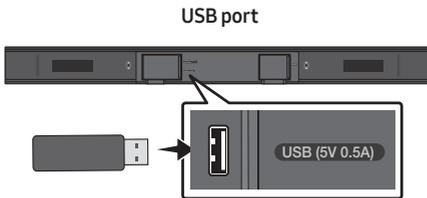
If an update is offered, you can update the firmware by connecting a USB device with the firmware update stored on it to the USB port on your Soundbar. For more information about how to download update files, go to the Samsung Electronics website at [www.samsung.com](http://www.samsung.com) → Support. Then, select the product type or enter the model number of your Soundbar, select the Software & Apps option, and then Downloads. Note that the option names can vary.
