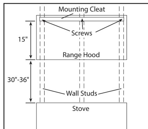
3. Rest the hood on the wood cleat with one person holding the hood. Score the drywall through at least 2 of the 3 holes located on the rear panel of the hood for placement of screws and/or drywall and anchors. Remove the hood and drill pilot holes into the marks transferred on the wall and add anchors if there is no stud(s) available.
