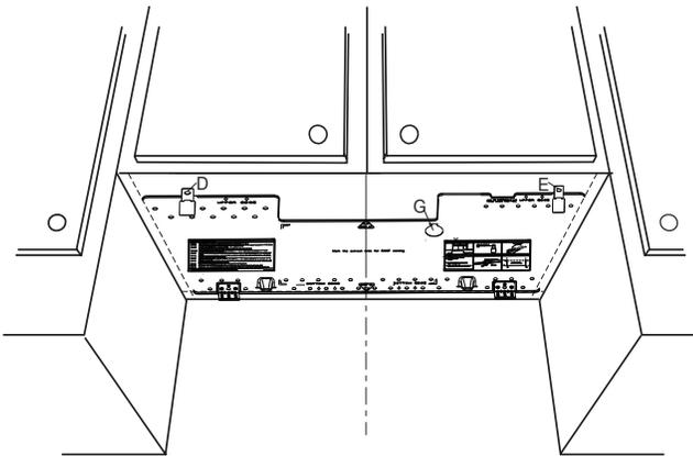
5. Cut the 1 1/2" (3.8 cm) diameter hole at the circular shaded area "G" on the template. This hole is for the power supply cord.
