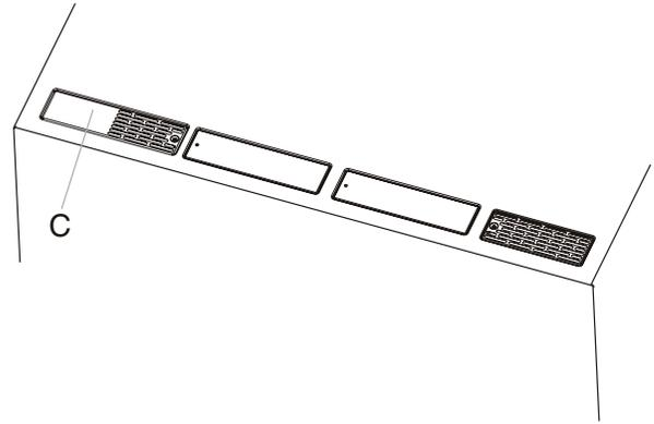
3. Remove the vent covers located in the upper polyfoam (see item J in "Parts Supplied" section).
