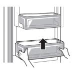
**2** To assemble the bin, slide it in above the desired support and push down until it snaps into place.
