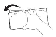
Remove the filter from the inside of the cover by pressing the side of the filter in and pulling the center out.
