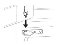
Fit the hinge ① over the hinge lever latch ② and slot it into place. Rotate the lever ③ clockwise and fasten the hinge.
