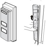
To remove the baskets, lift up and pull out.
