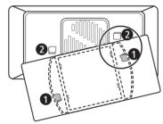
**5** Rotate the air filter cover clockwise until the hooks engage and the cover locks in place.
