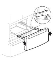
Lower the door into its final position and insert the screws in the rails on both sides.
