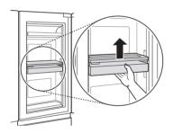
To lower the bin, press the side levers up at the same time and move the bin down until it clicks into place.
