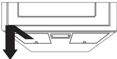
2. Soak the grease filter in hot water and a mild detergent. Rinse well and shake to dry. Brushing the filter lightly can remove embedded dirt.
