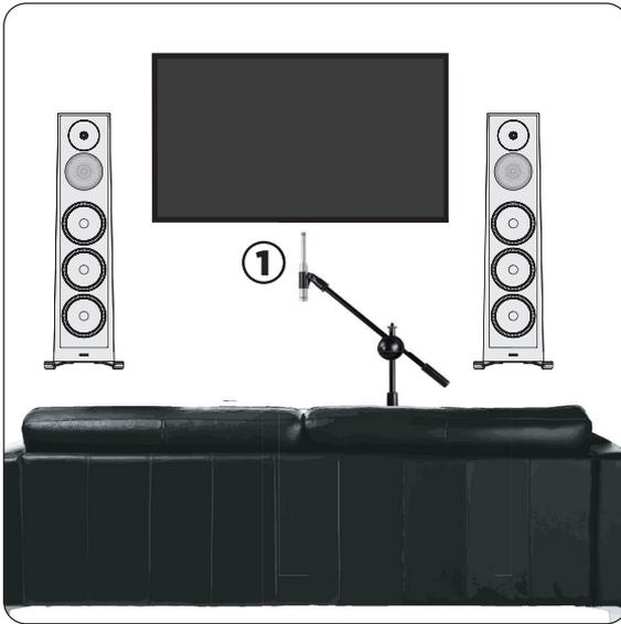
During all measurements, the microphone must point straight up.
