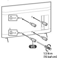
3 Attach the Wall-Mount Bracket (not supplied) using the screws (not supplied).
