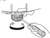
Open the door and check to make sure that the door closes easily.
