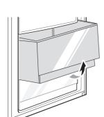
Press on the hook inside the top compartment, and then take out the air filter.
