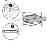
Tilt the drawer slightly and support it with one hand while pulling it out.
