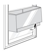
To reassemble, slightly tilt up the front, insert the crisper into the frame and push it back into place.
