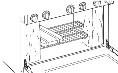
**CAUTION** Doors and passageways leading to the installation location require at least 32" opening. If the opening is less than 32", the oven door(s) and control knobs must be removed.
