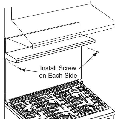
Install Screw in Top Corner on Each Side
