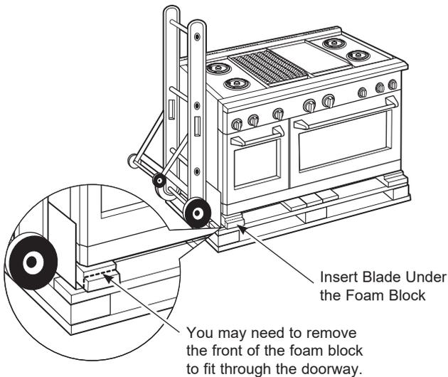
**IMPORTANT:** Do not remove the base foam block while the hand-truck is in use. Place the hand-truck blade underneath the base foam block and transport the range to the final location.
