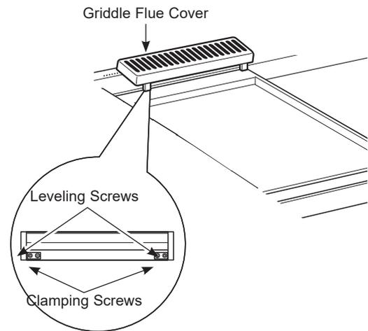
The two inner screws are clamping screws for securing the griddle in place. Loosen these two screws before leveling. Do not remove these two screws.
