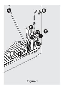
If you use braided flexible stainless steel tubing - The nut is already assembled on the tubing. Slide the nut onto the valve inlet and finger tighten the nut onto valve. Tighten another half turn with a wrench; DO NOT overtighten. See Figure 2.
