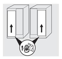
After leveling, verify the door stop contacts the lower hinge and the top of the door does not contact the upper hinge through full movement of the door (from fully closed to fully open).
