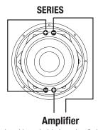
Series wiring a dual 1 ohm sub = 2 ohm
