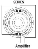
Series wiring a dual 2 ohm sub = 4 ohm
