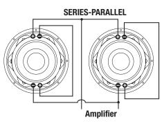
Series-Parallel wiring two dual 1 ohm subs = 1 ohm
