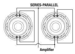
Series-Parallel wiring two dual 2 ohm subs = 2 ohm
