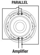
Parallel wiring a dual 2 ohm sub = 1 ohm
