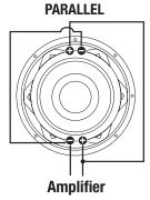
Parallel wiring a dual 1 ohm sub = 1/2 ohm
