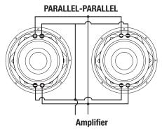
Parallel-Parallel wiring two dual 1 ohm subs = 1/4 ohm
