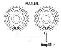
Parallel wiring of two single 4 ohm subs = 2 ohms
