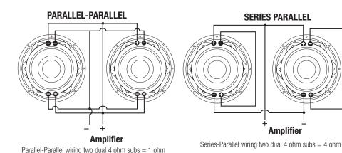
NOTE: Never connect only one coil of a Dual Voice Coil (DVC) speaker. BOTH voice coils must be connected to the amplifier
