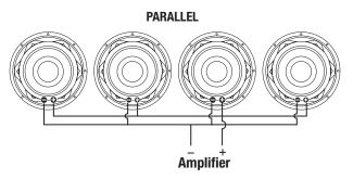
Parallel wiring of four single 4 ohm subs = 1 ohms
