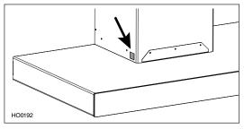
2.Carefully slide in place decorative lower flue (notches end first) on top of the hood (1) until flue notches completely fit in hood slots (2).
