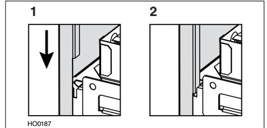
Slide up the upper flue until it is aligned with its mounting bracket. The bracket must be inside the flue. Secure the upper flue to its bracket using 2 no. 8 x 3/8" screws for stainless steel model or 2 no. 8 x 1/2" quadrex black screws for black stainless steel model (included). See illustration beside.
