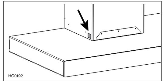
2. Carefully slide in place decorative lower flue (notches end first) on top of the hood (1) until flue notches completely fit in hood slots (2).
