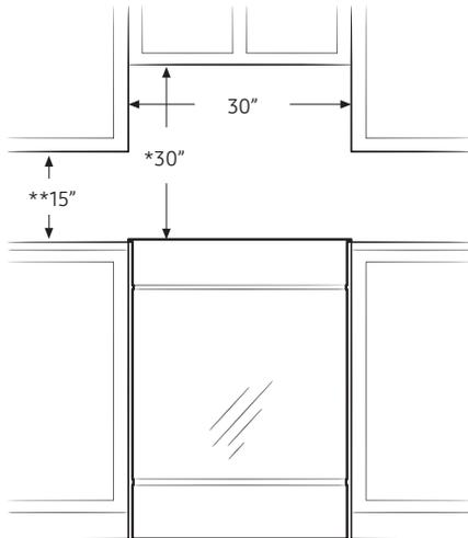
\* A minimum of 30" is required between the top of the cooking surface and the bottom of an unprotected wood or metal cabinet; a minimum of 24" is required if the bottom of the wood or metal cabinet is protected by not less than 1/4" of flame retardant millboard covered with not less than no.28 MSG of sheet steel, 0.015" of stainless steel, 0.024" of aluminum, or 0.020" of copper.
