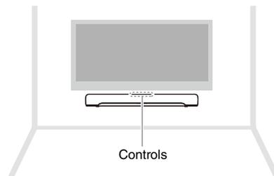
Refer to the User Guide. When installation and all connections are complete, power off sound bar and hold down BASS EXT on the sound bar's remote control for at least five seconds. The frequency characteristics are configured for wall mount installation.
