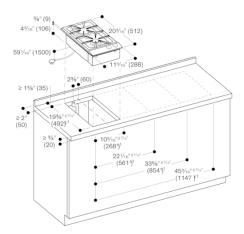
Minimum distance from the appliance cut-out to the side wall 11<sup>13</sup>/<sub>"0</sub>" (300 mm), measurements in inches (mm)
