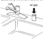
that the drain hose either be looped up and securely fastened to the underside of the counter.or be connected to an air gap. Make sure to use an air gap if the drain hose is connected to house plumbing lower than 20" (50.8 cm) above subfloor or floor.
