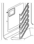
Slide the rear prongs of the side rack back into the holes, ensuring the rack is firmly pushed up against the side wall of the oven.
