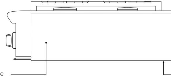
The rating label is located on the right-hand side of the rangetop, near the front.
