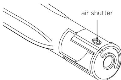
Each valve and air shutter is individually tested and adjusted prior to shipment. Normally adjustment is not required, however, vibration during transit, gas conversion or variations in the local gas supply may make minor adjustments necessary.
