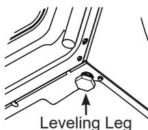
**NOTE: Keep the leg extension at a minimum to prevent excessive vibration. The farther out the legs are extended, the more the washer will vibrate.**
