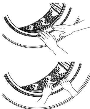
Remove any foreign objects if found trapped inside this gasket. Make sure there is nothing blocking the holes behind the gasket.
