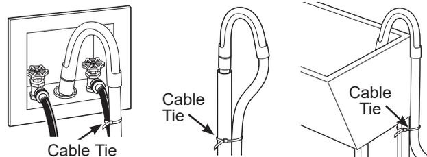
**NOTE:** Placing the drain hose too far down the drain pipe can cause a siphoning action. No more than 7 inches of hose should be in the drain pipe. There must be an air gap around the drain hose. A snug fit can cause a siphoning action.
