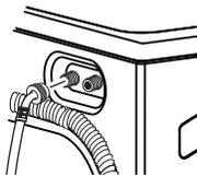
4. If inlet hose screen washers are not already inserted into the inlet hoses, install them by inserting into the free ends of the HOT and COLD inlet hoses with protruded side facing the faucet.
